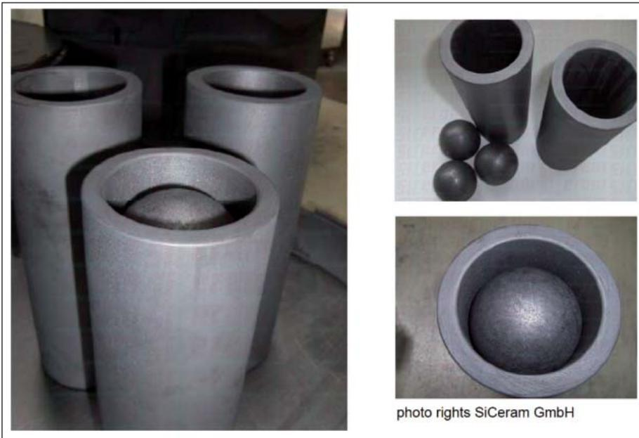
Fig. 8. SiC pilot canister with 3 graphite pebbles, overall dimensions:  $D \approx 82 \text{ mm}$ ;  $H \approx 205 \text{ mm}$ .
